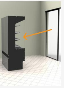
A location near a doorway will affect the airflow and holding temperature of open and closed showcases.
