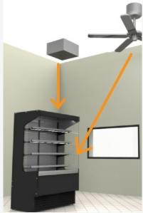
HVAC ceiling vents and ceiling fans will affect the airflow of open showcases and could create condensation on the glass of closed showcases.
